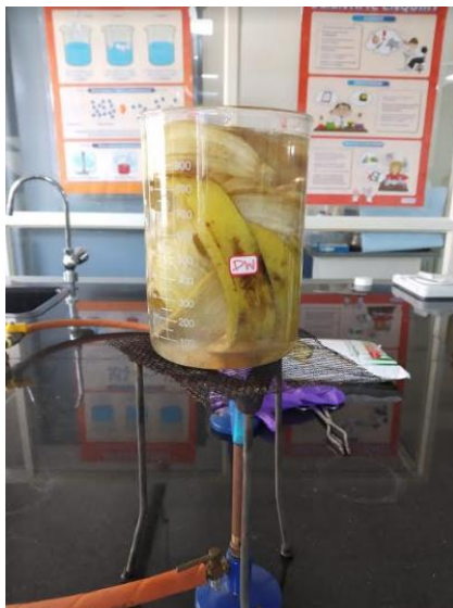
Figure 2: Placing the peels in boiling water over a tripod stand and Bunsen burner.
