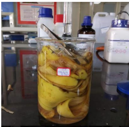
Figure 1: Soaking the peels in sodium thiosulfate.
