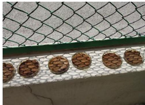
Figure 4: Drying the plastic samples in the sun.
