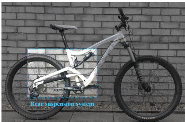
Figure 1: A mountain bike with a rear suspension system (highlighted).
