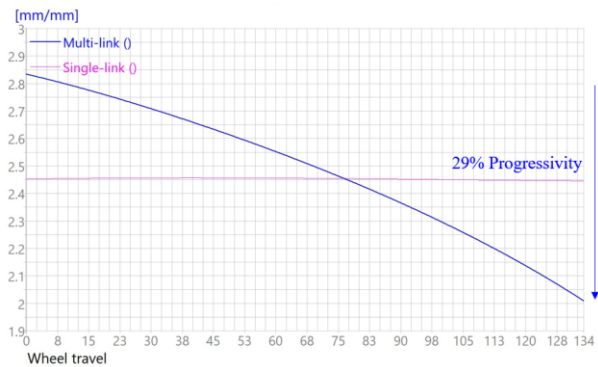
Figure 16: Leverage curves comparison from Linkage X3.
